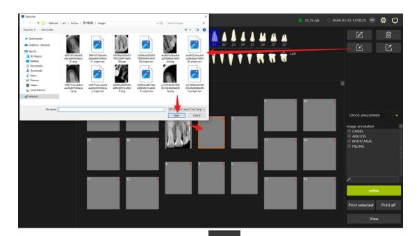
a) Select an empty rectangle and click Import to open the file selection interface. The imported file supports DCM, raw, BMP, JPG, JPEG and PNG formats; After successful import, the imported image displays normally;
