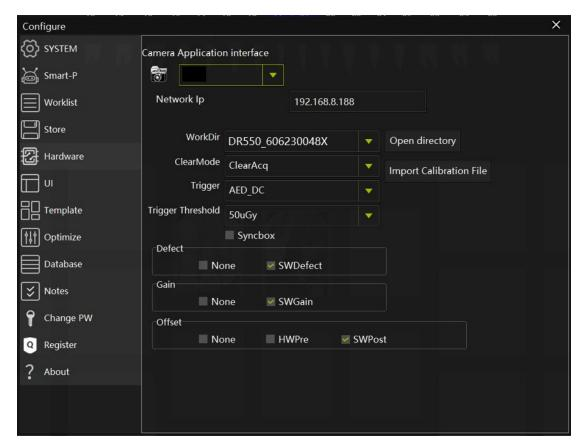
**Camera application interface:** the default is test, which is actually used according to the application scenario;
